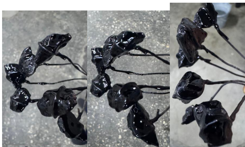
Figure 2. Binding of bitumen with inert material
