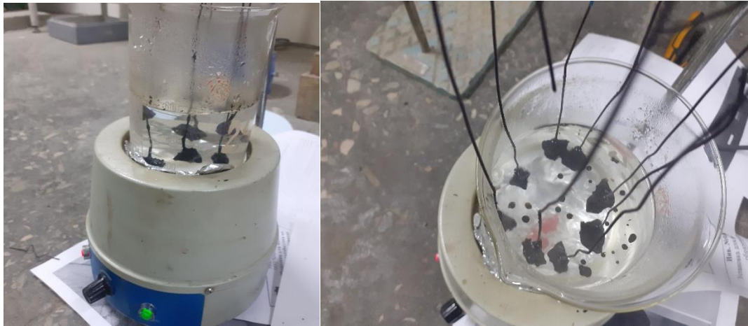
Figure 1. Boil the prepared sample in water for 30 minutes.
